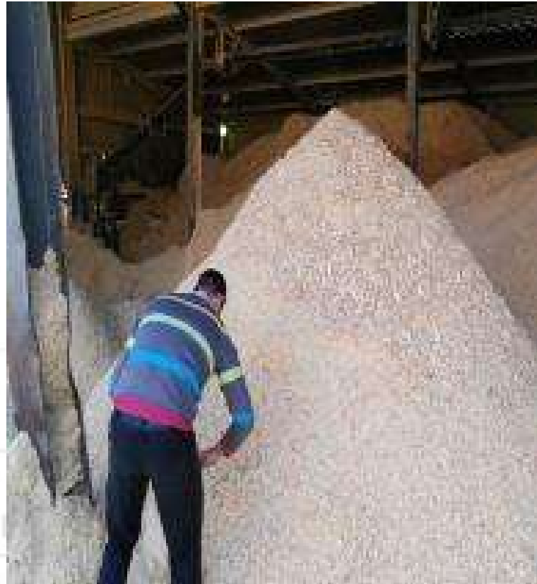
Collection of clean uncontaminated sawdust in basement of sawmill during the sawmilling operation
