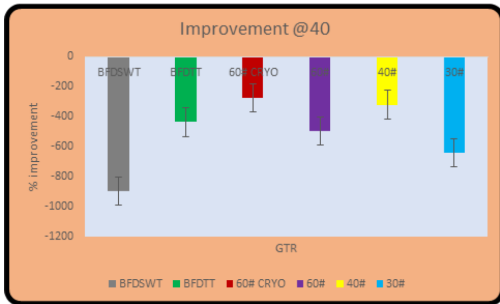
Figure 3.2.2.2 A: 3-point bend improvement at 40 % GTR contents at ambient temperatures.
