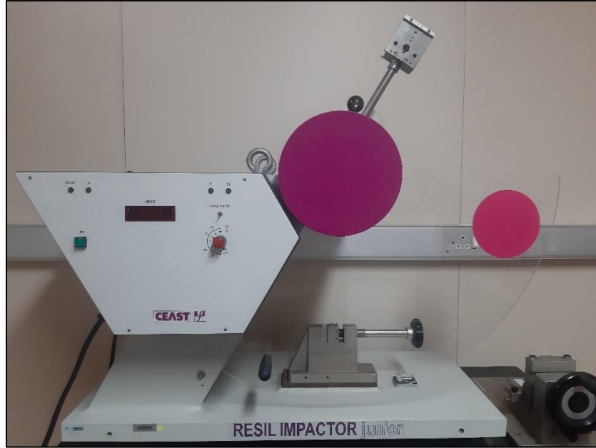
Figure 2.4: A photograph of the Resil Impactor junior used in the study.
