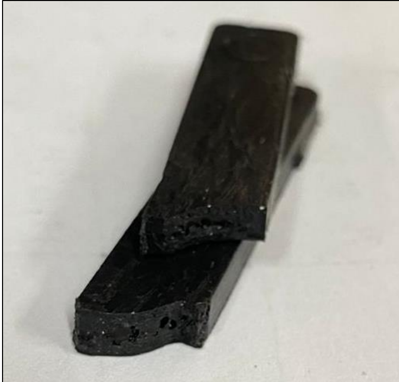
Figure 2.3.2.2 A: A photograph of an Impact Resistance break sample used for failure analysis using SEM.
