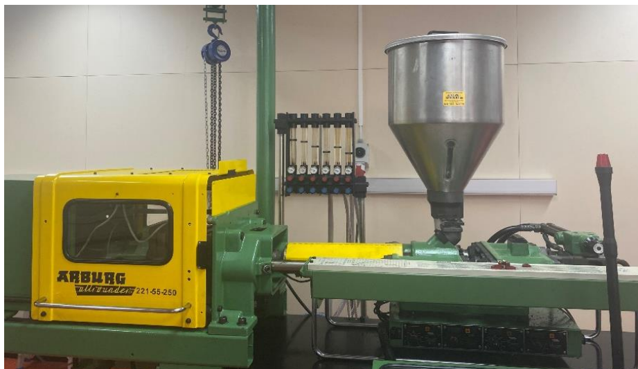
Figure 3.4: ARBURG 221-55-250 reciprocating screw Injection Moulder.
