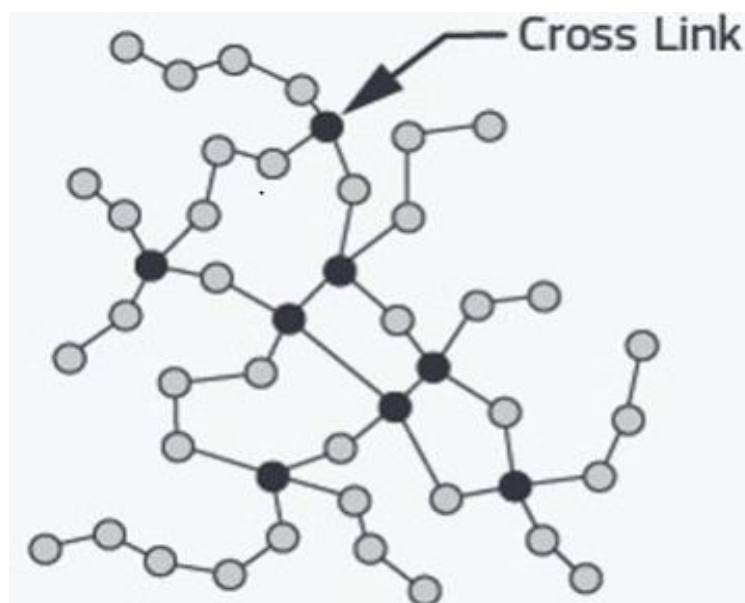
Figure 2.4: Molecular alignment of thermosetting plastics [14].
