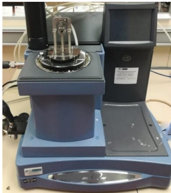
Figure 3.9: A picture of the TA-Instruments' DMA Q800 used in this study
