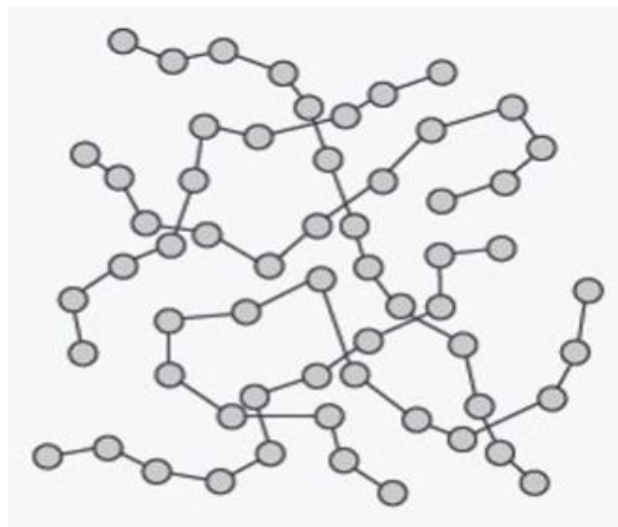
Figure 2.5: Molecular alignment of thermoplastics [18].
