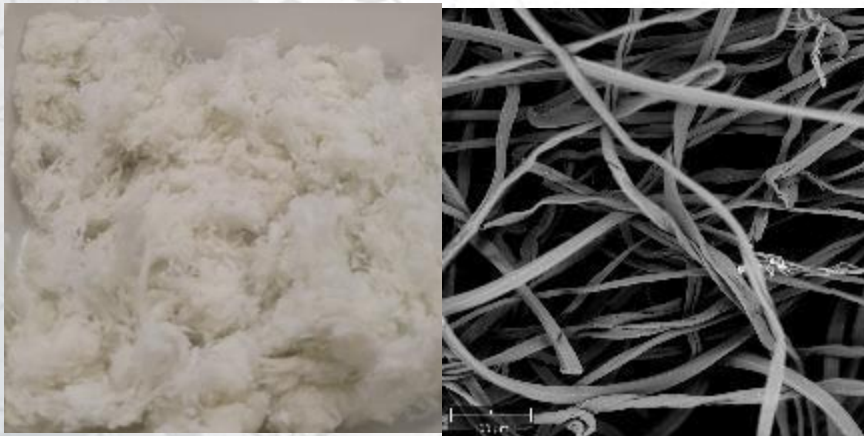
Figure 1: Visual appearance (left) and SEM-micrographs (right) of decolourised materials a) woven fabric waste [ b) knitted fabric waste and c) mixed shoddy waste
