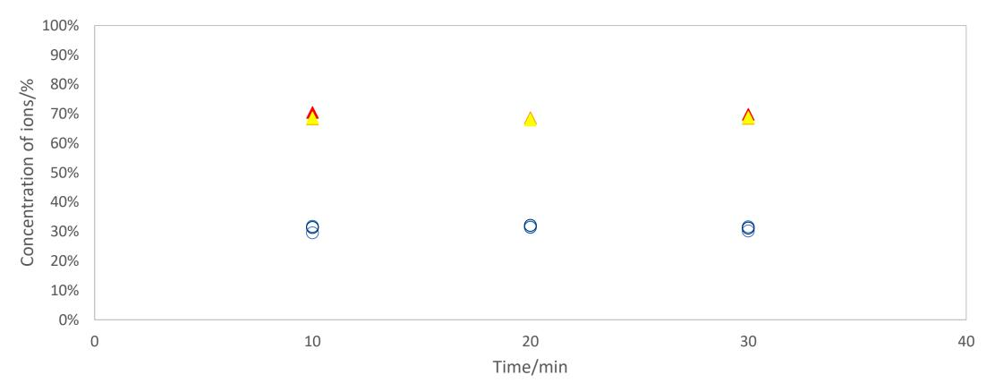
Concentrations of Fe<sup>3+</sup> (  $\land$  2.2M HNO<sub>3</sub>,  $\land$  6.7M HNO<sub>3</sub>,  $\land$  12.3M HNO<sub>3</sub> ) and Nd<sup>3+</sup> ( $\circ$  2.2M HNO<sub>3</sub>,  $\circ$  6.7M HNO<sub>3</sub>,  $\circ$  12.3M HNO<sub>3</sub>) ions in the pregnant leach solution of acid concentration test. Particle size = 425-500 µm, T = 298.15 K, t = 30 min.
