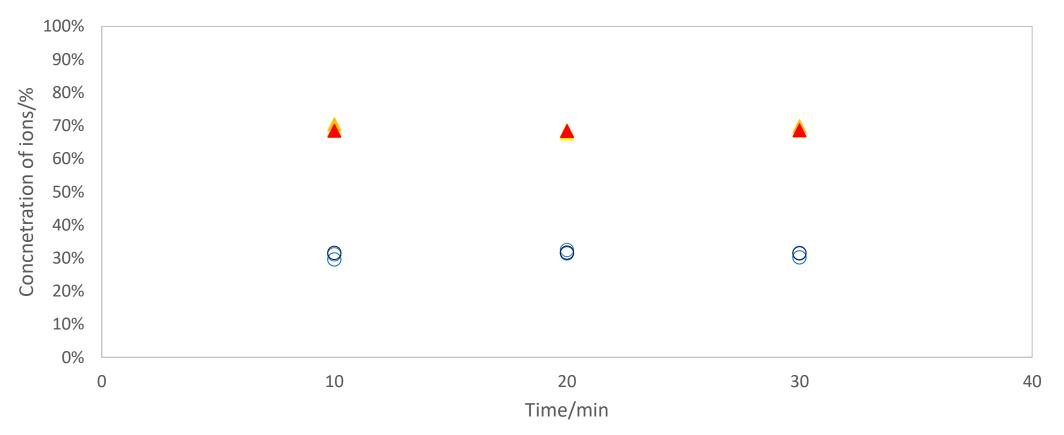
Concentrations of Fe<sup>3+</sup> (  $\land$  100-150µm,  $\land$  425-500µm,  $\land$  ≥600µm ) and Nd<sup>3+</sup> ( $\circ$  100-150µm,  $\circ$  425-500µm,  $\circ$  ≥600µm ) ions in the pregnant leach solution of particle size test. 2.2M HNO<sub>3</sub>, T = 298.15 K, t = 30 min.
