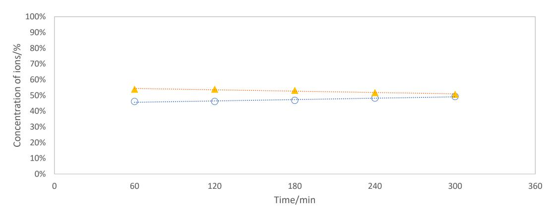
Concentrations of Fe<sup>3+</sup> ( $\blacktriangle$ ) and Nd<sup>3+</sup> ( $\circ$ ) ions in the pregnant leach solution of contact time test. Particle size = 425-500 µm, 12.3M HNO<sub>3</sub>, T = 298.15 K.
