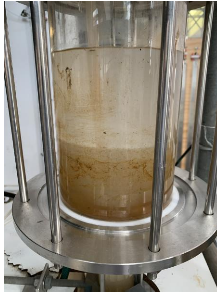
Figure 3-6: Top settling tank
