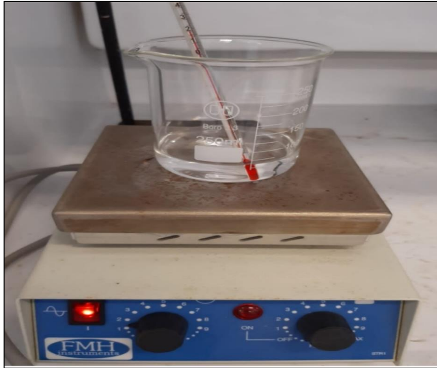
Figure 3.3. The magnetic stirrer apparatus containing two dials. The dial on the left controls the magnetic stirrer speed, and the dial on the right controls temperature
