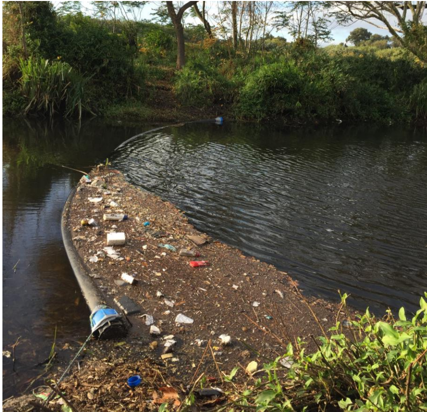
Figure 2. A litterboom installed by an NGO on the Liesbeek River, Cape Town as part of a Dutch-South African research collaboration.
