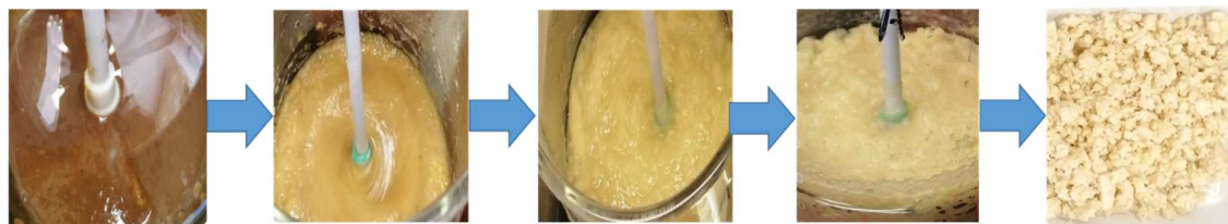
Figure 4: Transition of sawdust to pulp during delignification process.
