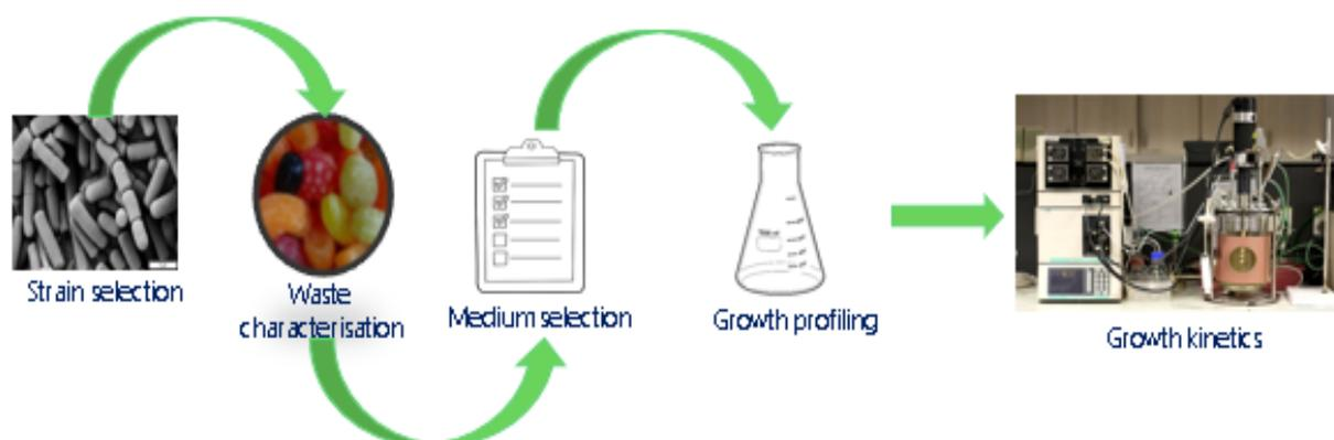
Figure 7-2 Experimental approach to investigating production of PGA from confectionery waste
