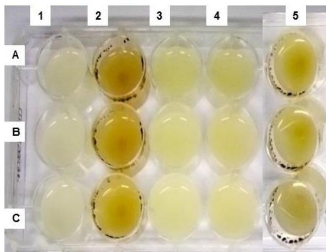
Figure 7-4 Multiwell plates containing 1) glucose, 2) chocolate, 3) hard candy, 4) marshmallow, and 5) the mixture after 30 h cultivation
