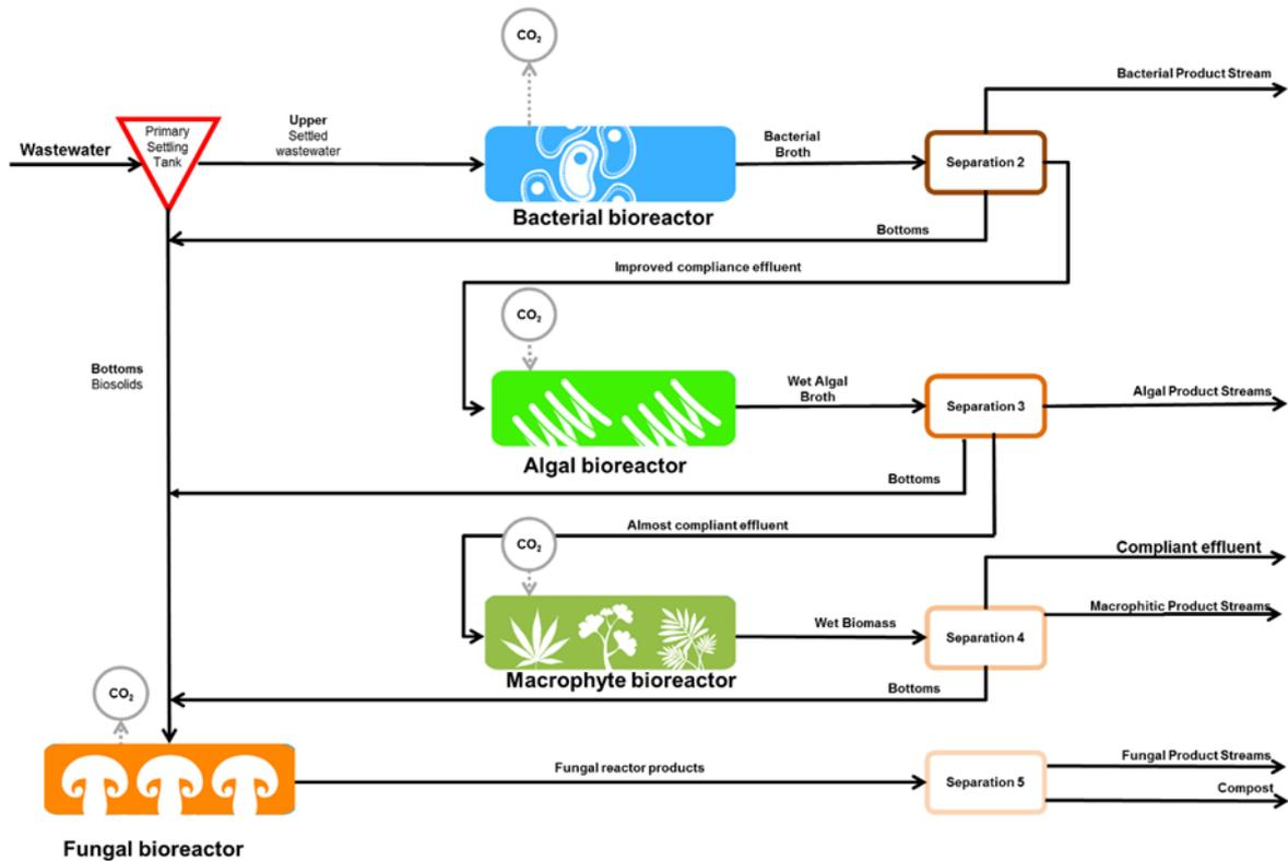
Figure 3-3 Overview of a wastewater biorefinery (Susan T. L. Harrison et al., 2017) Current South African research on “Waste to Energy” (WtE)
