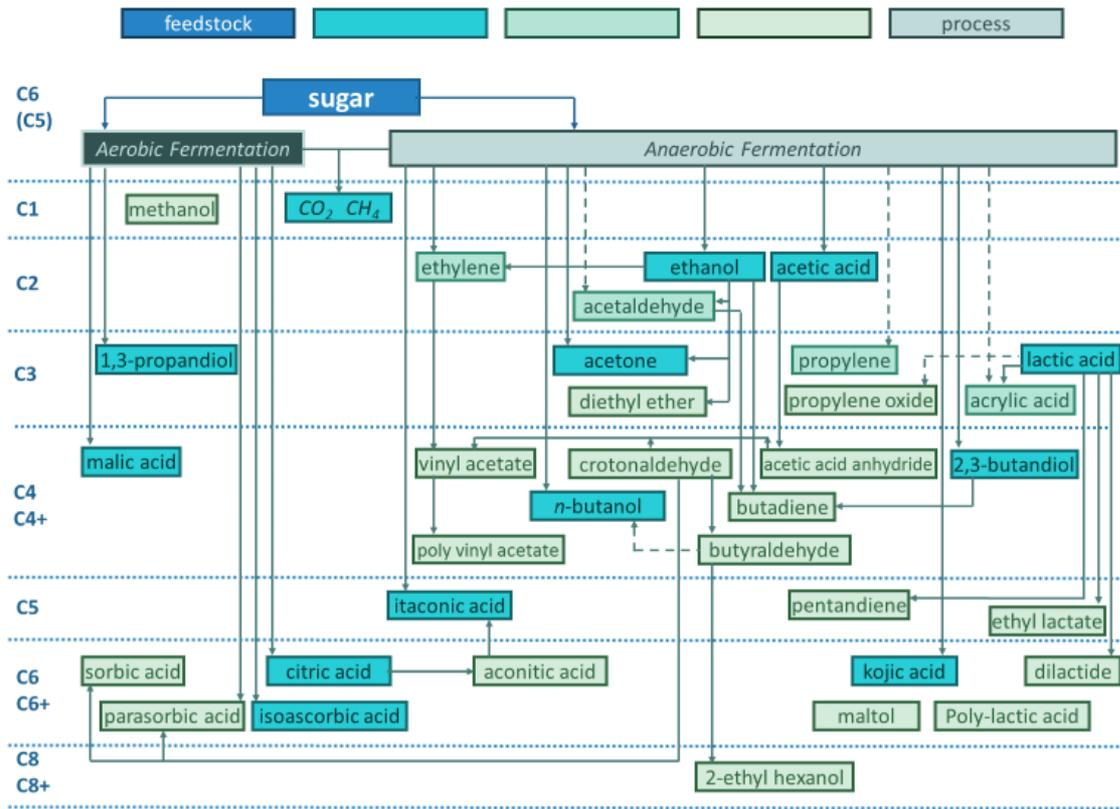
Figure 3-4 Various biobased chemicals that can be produced from the aerobic and anaerobic fermentation of sugar: after Kamm et al. (2010)
