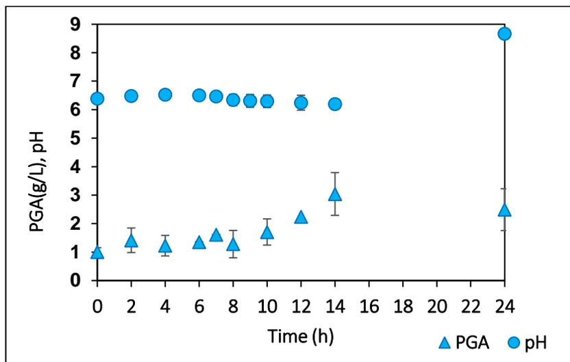
Figure 7-16 pH profile and PGA formation on hard candy waste. (PGA concentration is given as (▲) while pH is given as (●))
