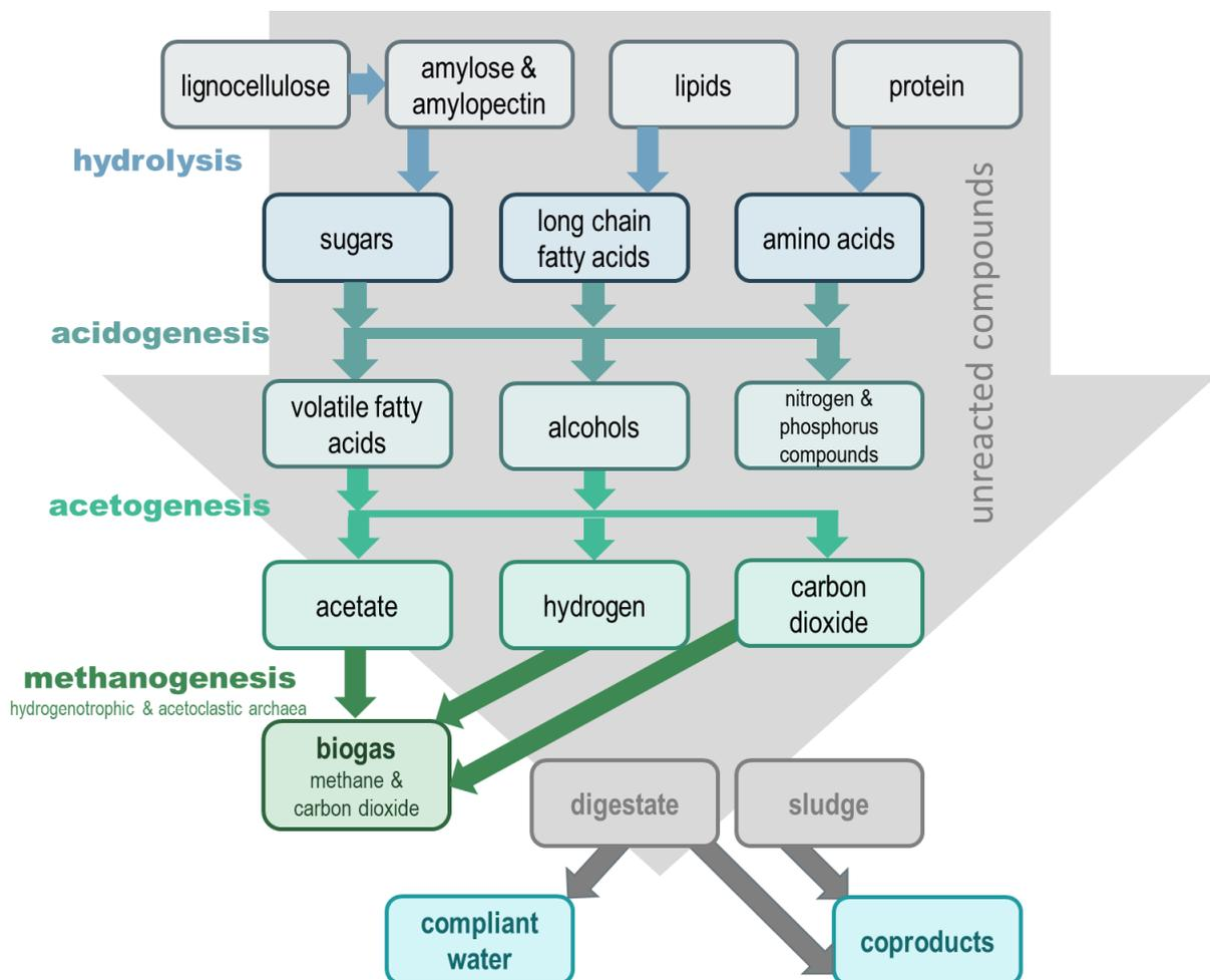
Figure 5-1 The four stages of the process of anaerobic digestion: adapted from Harrison et al. (2019)
