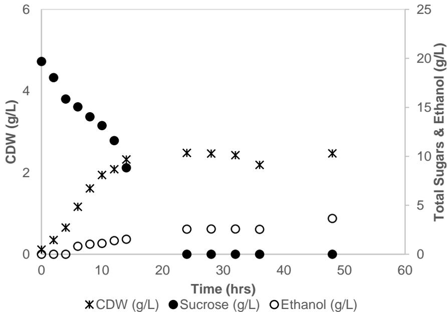
Figure 5-12 Growth and ethanol production by *Z. mobilis* on synthetic sugar mix as carbon source in New Brunswick bioreactors at 30°C. Data represents the averages of two replicate bioreactor fermentations
