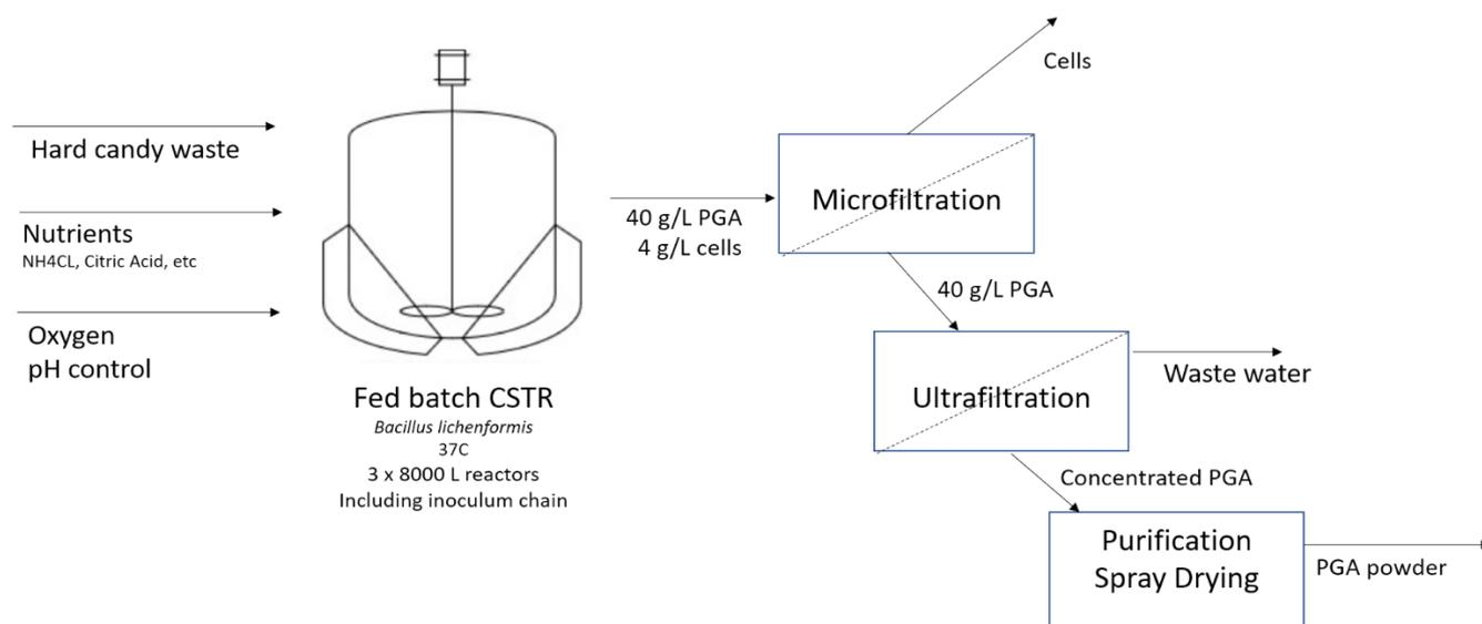
Figure 9-1 Simplified PGA production flowsheet
