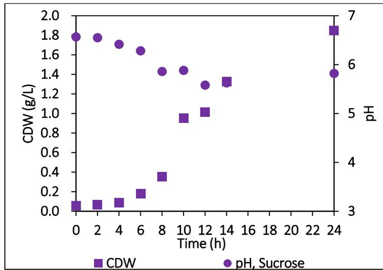
Figure 7-7 Growth of *B. licheniformis* on sucrose in shake flasks (pH is given as (●) while biomass concentration is given as (■))
