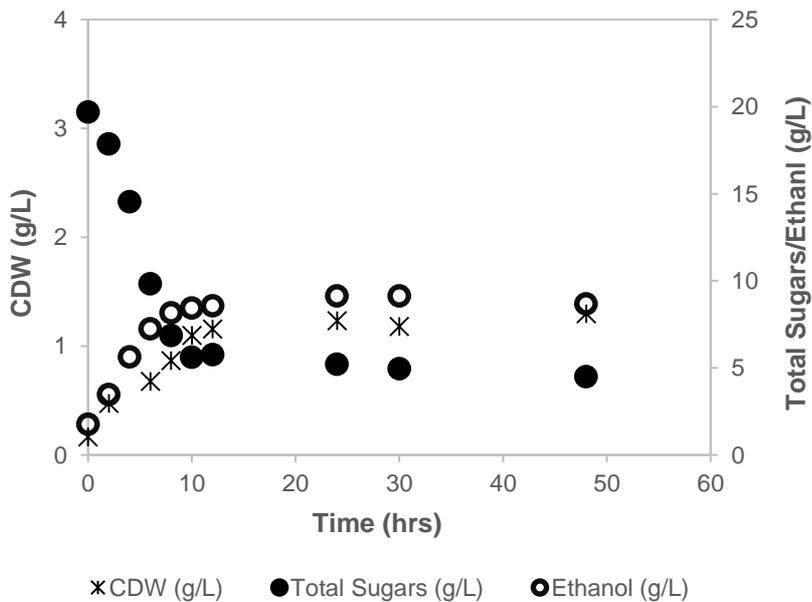
Figure 5-17 Growth and ethanol production by *Z. mobilis* fermentations performed with chocolate as substrate in large scale bioreactors. Data represent the averages of two replicate fermentations.
