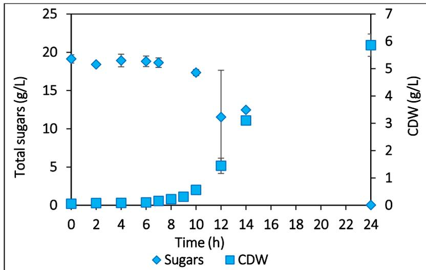
Figure 7-15 Growth of *B. licheniformis* and associated sucrose utilisation when grown on hard candy waste at pH 6.5, aeration 1 vvm and 37 °C with agitation starting at 500 rpm. Total sugar concentration is given as (◆), while biomass concentration is given as (■).
