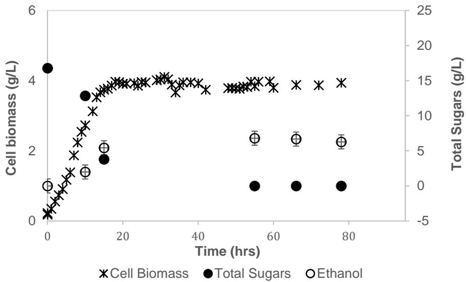
Figure 5-6 Growth, sugar utilisation and ethanol production from small-scale fermentation studies of *Z. mobilis* cells on synthetic sugar mix as carbon source following pre-exposed of the inoculum to sucrose. Data points represent the average of results obtained from three independent experiments with error bars indicating standard deviation
