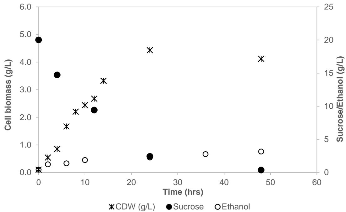
Figure 5-8 Growth, sugar utilisation and ethanol production from small-scale fermentation studies of *Z. mobilis* cells on chocolate as carbon source following pre-exposed of the inoculum to sucrose. Chocolate studies were conducted in duplicate.
