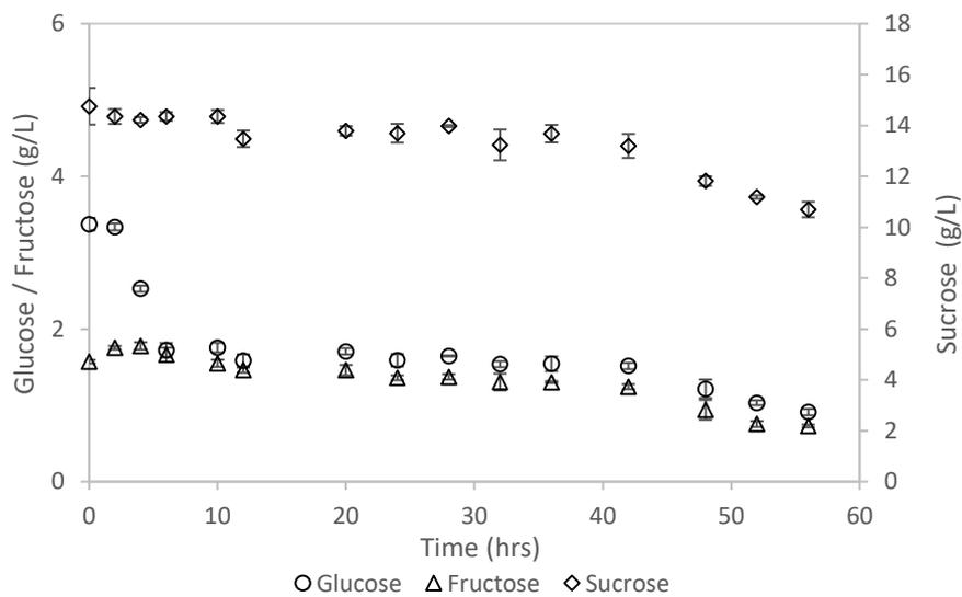
Figure 5-3 Utilisation of individual sugars contained within hard candy confectionery during *Z. mobilis* fermentation. Data points represent the average of results obtained from three independent experiments with error bars indicating standard deviation.
