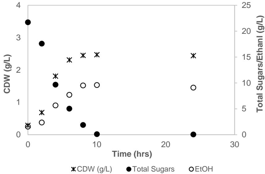
Figure 5-13 Growth and ethanol production by *Z. mobilis* on sucrose as carbon source in New Brunswick bioreactors at 37°C. Data represents the averages of two replicate bioreactor fermentations.
