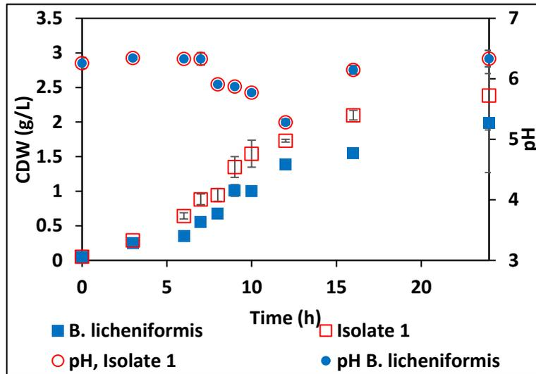
Figure 7-11 Cultivation of Isolate 1 and *B. licheniformis* on dextrin in shake flasks
