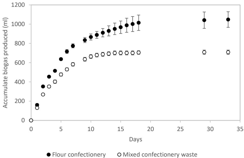
Figure 5-18 Total biogas production from the anaerobic digestion of flour confectionery and mixed confectionery feedstocks. Data points indicate the average of three independently performed BMP tests and the error bars indicate standard error.
