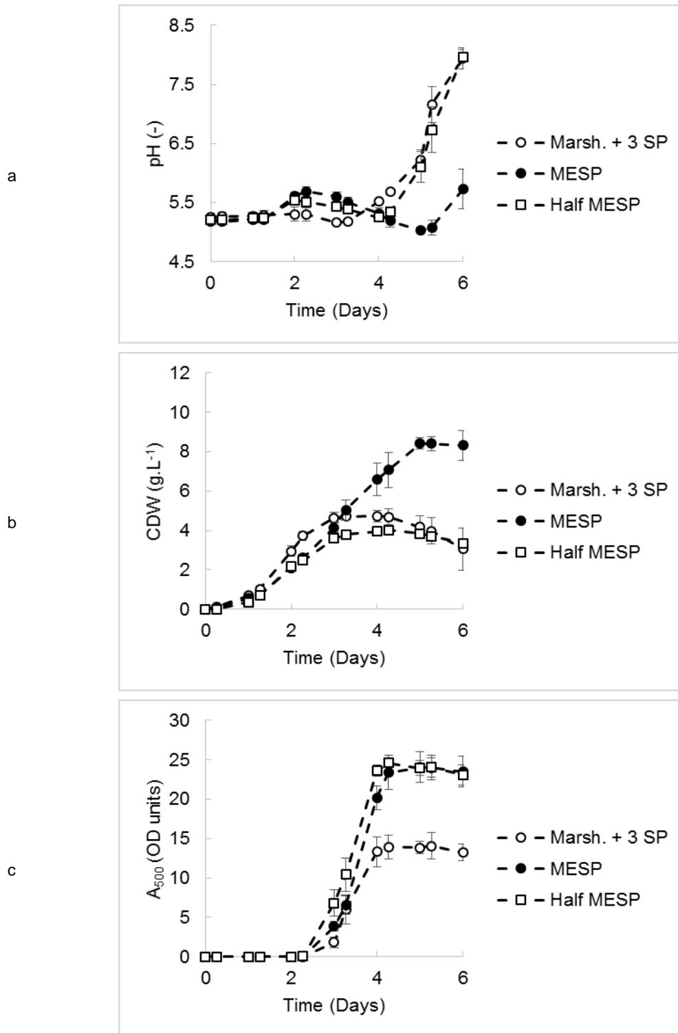
Figure 8-7 Comparison of the pH trends (a), growth (b) and pigment production (c) when cultivating *P. purpurogenum* in the BioFlo 110 fermentor at 30 °C, using Marsh. + 3 SP, MESP or Half MESP medium, all maintained at a pH of 5 through application of a 50 mM citrate buffer. Results show the average of triplicate measurements during duplicate cultivations, with error bars representing standard deviation of the data.
