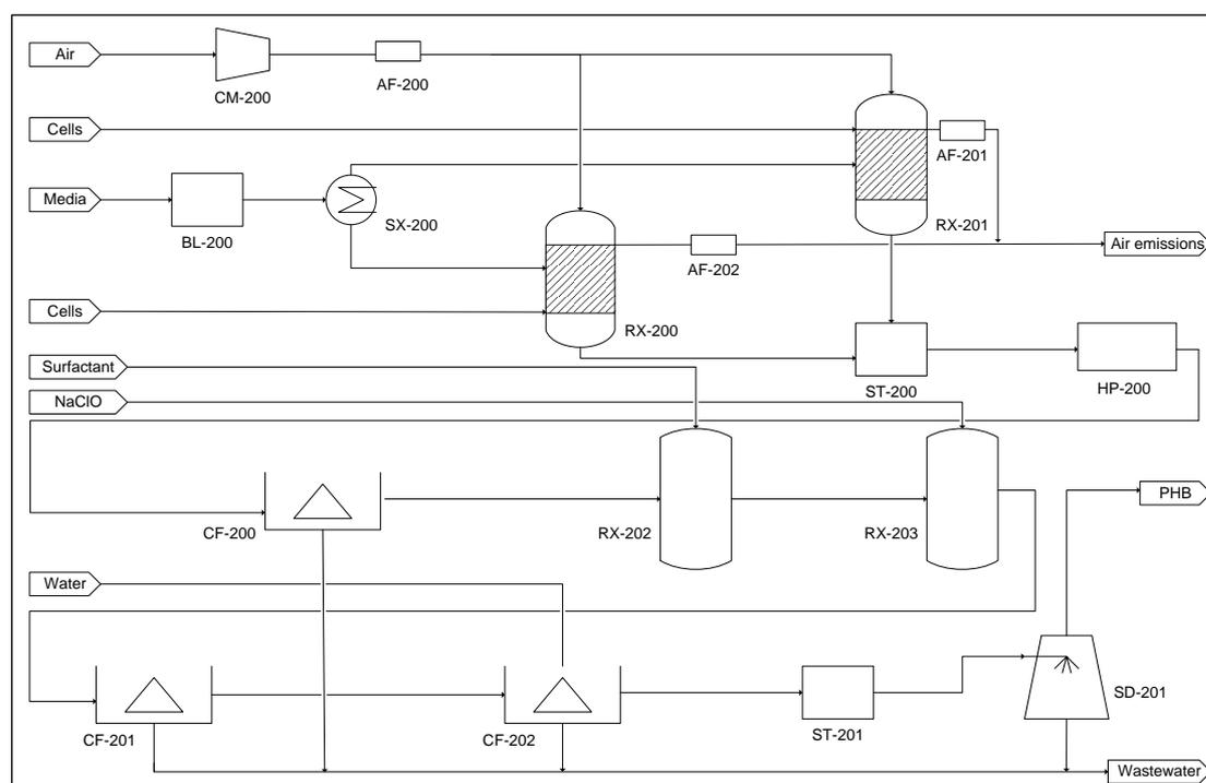
Figure 6-5 Process flow diagram for the production of PHB using in the CeBER Bioprocess Modeller simulation (adapted from Rumjeet and Harrison, in prep b). Key: SX-200 – steam steriliser, RX-200 and RX-201 – bioreactor, CM-200 – compressor, HP-200 – high pressure homogeniser, CF-200 and CF-201 – centrifuge, RX-202 – DSP reactor 1, RX-203 – DSP reactor 2.
