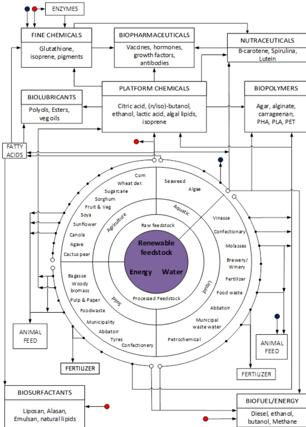
Figure 3-2 Linking potential bioproducts with raw materials from which they may be manufactured (Harrison et al., 2016), thereby providing insight into the potential diversity of biorefinery products
