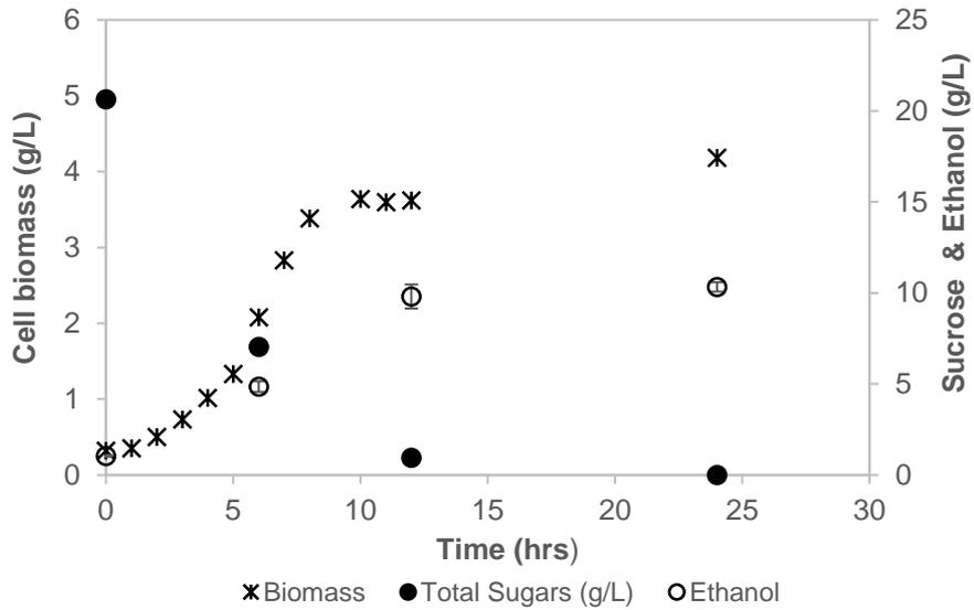
Figure 5-4 Growth, sugar utilisation and ethanol production from small-scale fermentation studies of *Z. mobilis* cells on sucrose as carbon source following pre-exposed of the inoculum to sucrose. Data points represent the average of results obtained from three independent experiments with error bars indicating standard deviation.
