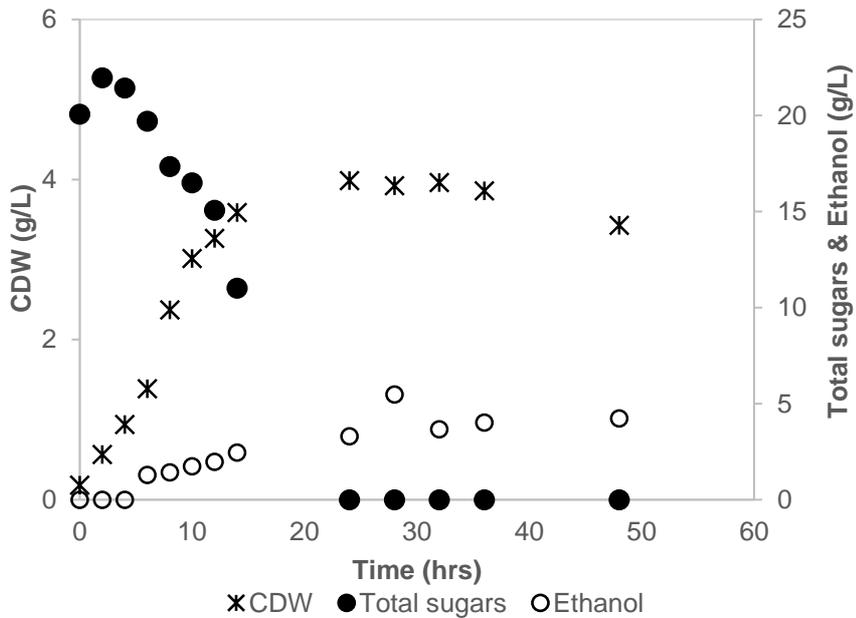
Figure 5-11 Growth and ethanol production by *Z. mobilis* on sucrose as carbon source in New Brunswick bioreactors at 30°C. Data represents the averages of two replicate bioreactor fermentations
