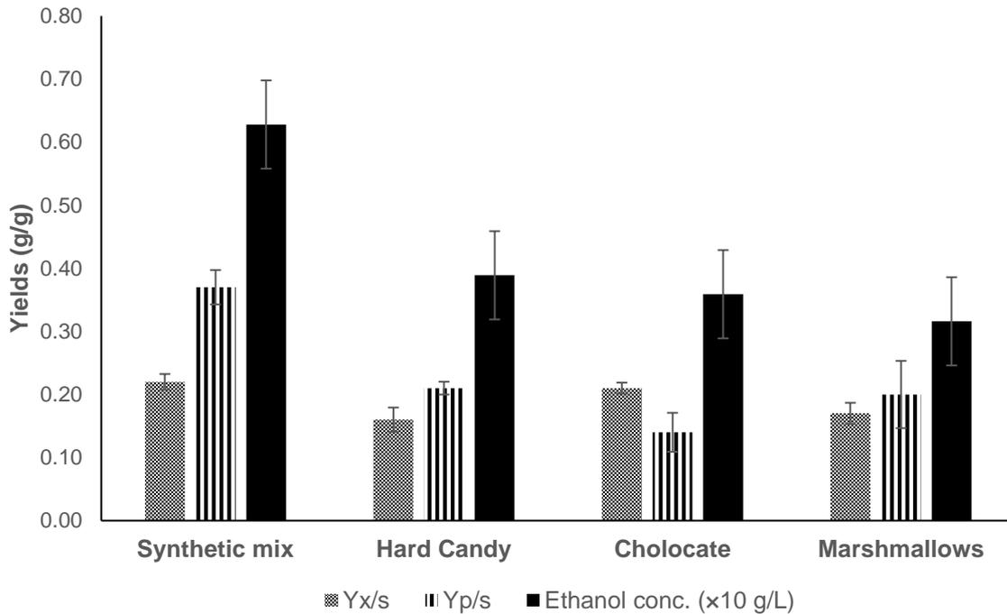
Figure 5-9 Biomass ( $Y_{x/s}$ ) and bioethanol product ( $Y_{p/s}$ ) yield coefficients and bioethanol concentrations achieved by *Z. mobilis* fermentations on various confectionery products and a synthetic sugar mixture simulating hard candy (10 g/L sucrose, 2.5 g/L glucose and 2.5 g/L fructose).
