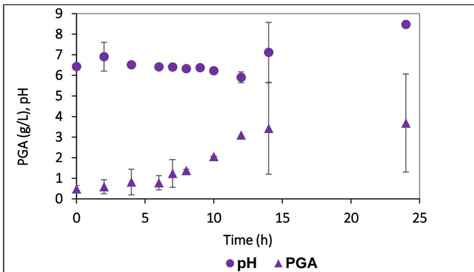
Figure 7-13 PGA formation and pH of a *B. licheniformis* culture grown in sucrose at pH 6.5, aeration at 1 vvm and 37 °C with agitation starting at 500 rpm. (PGA concentration is given as (▲), while pH is given as (●))
