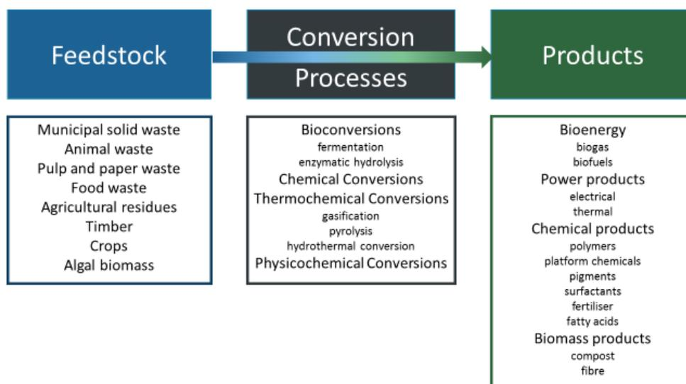
Figure 3-1 Schematic diagram of a biorefinery process (based on Fernando et al. (2006))
