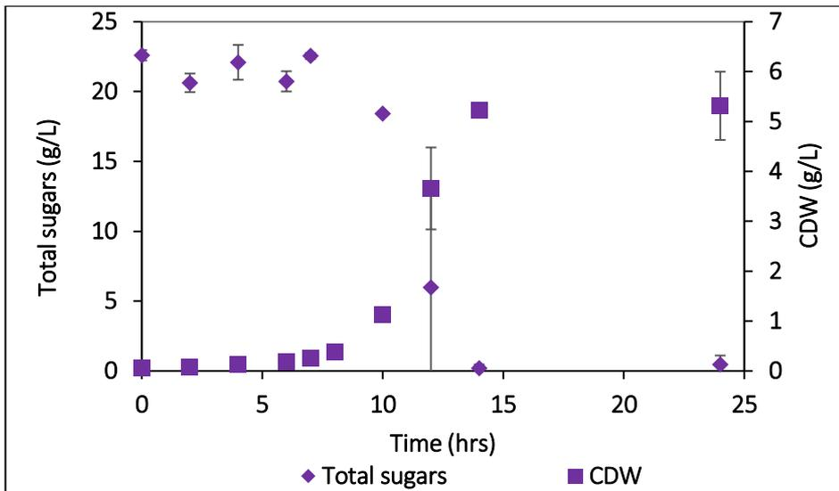
Figure 7-12 Sugar utilisation of *B. licheniformis* on sucrose at pH 6.5, aeration at 1 vvm and 37 °C with agitation starting at 500 rpm. (Biomass concentration is given as (■) and total sugars given as (◆))
