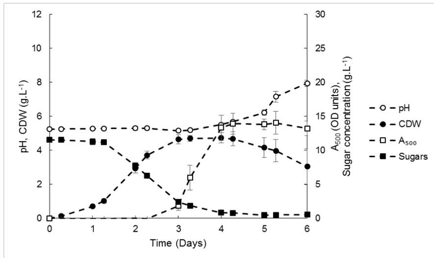
Figure 8-5 Summary of cultivation of *P. purpureogenum* DSM 62866 on Marshmallow + 3 SP medium, pH 5 (50 mM citrate buffer), at 30 °C in the BioFlo 110 modular benchtop fermentor for 6 days. The average pH, growth, pigment production, and sugar concentration for triplicate measurements performed during duplicate cultivations are shown, with error bars representing the standard deviation of the data.
