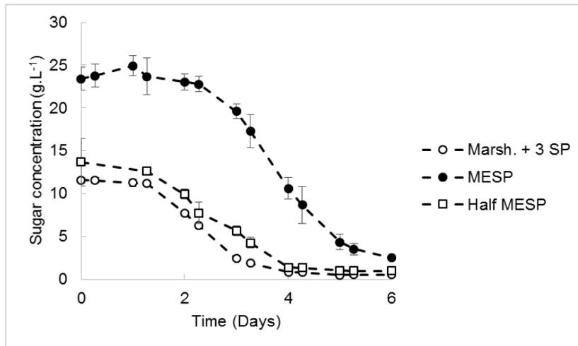
Figure 8-8 Comparison of sugar utilization trends in the BioFlo 110 fermentor using either marshmallow- or malt extract-based cultivation media. Results represent the average of triplicate measurements during duplicate cultivations. Error bars show the standard deviation of the data.
