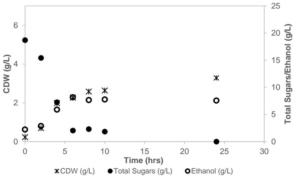
Figure 5-14 Growth and ethanol production by *Z. mobilis* on synthetic sugar mix as carbon source in New Brunswick bioreactors at 37°C. Data represents the averages of two replicate bioreactor fermentations.
