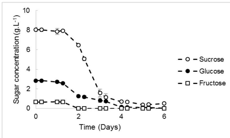
Figure 8-6 Concentration of individual sugars during BioFlo 110 cultivation of *P. purpureogenum* on marshmallow medium supplemented with 3 g/L soya peptone, pH 5, 50 mM citrate buffer at 30 °C, determined using HPLC analysis. Error bars represent the standard deviation associated with triplicate measurements across duplicate cultivations.
