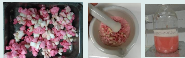
Figure 4 Making marshmallow into substrate for microorganisms
