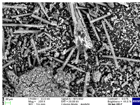
Figure 1. Scanning Electron Microscope Image of PCB residue
